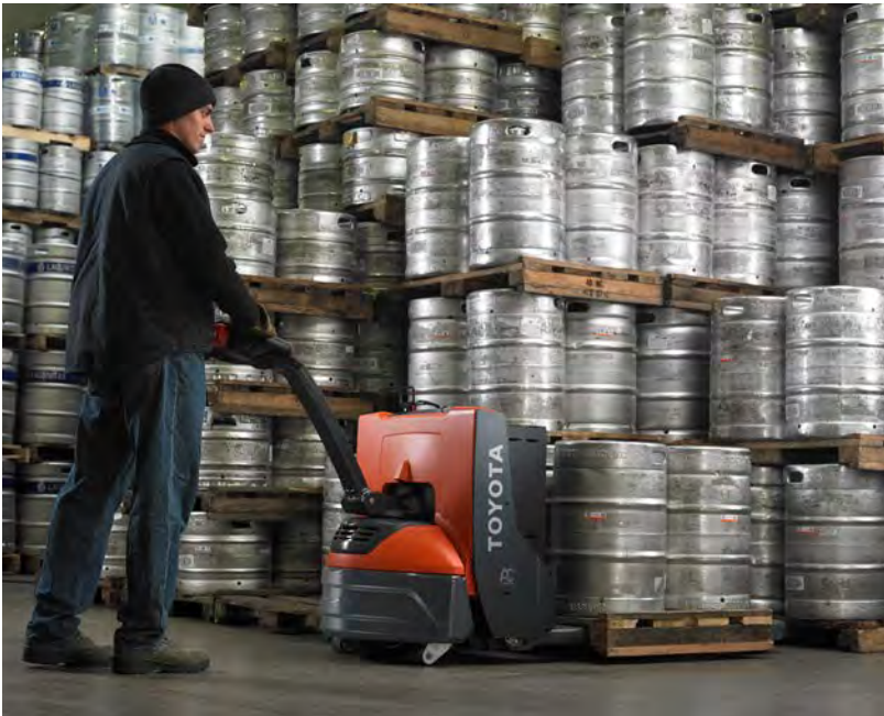
The Toyota electric walkie pallet jack is a popular model used in cold storage operations because of its maneuverability in tight spaces.
